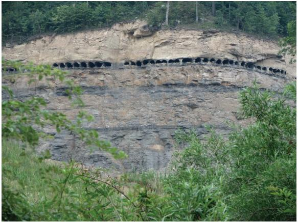
Auger mining in the Pikeville Formation in Knott County. Auger mining is usually associated with contour strip mining. The coal is removed by drilling auger holes from the last contour cut and extracting it in the same manner that shavings are produced by a carpenter's bit. Coal recovery rates approach 60 percent. The cutting heads of some augers are as large as 8 feet. Augers can penetrate up to 1000 feet into the mountainside. Photo by Dan Carey, Kentucky Geological Survey.
